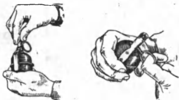
48-rasm. Zapalni burab o'rnatish va saqlovchi tortiqni sug'urish.
