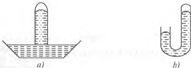
1.1-rasm. Simobli barometr: a) idishli, b) sifonli.
