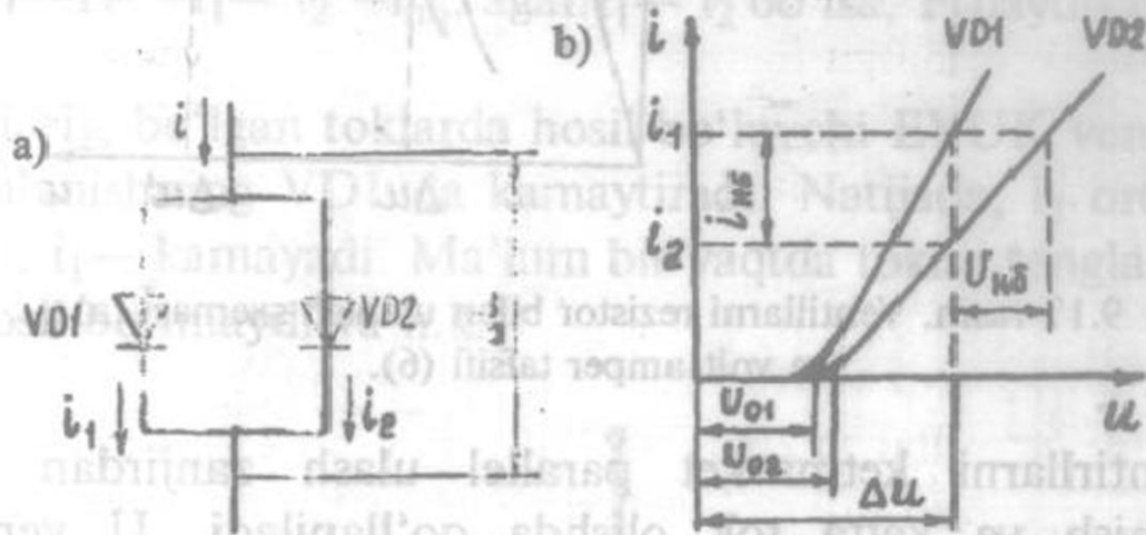
9.16-rasm. Ventillarni parallel ulash sxemasi (a) va ularning gurri volt-ampere tavsiflari (b).
